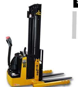
Brake is applied when control arm is in the vertical or horizontal handle position. Travel speed is reduced when forks are above 12" fork height. Position hold resists roll back on ramps.
